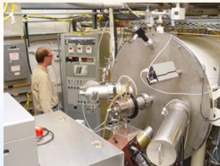
Danny Crews, systems engineer for instrumentation and controls at the Space Chambers research lab, checks pressure readings on the pumping system control rack to the left of the CCOSE Chamber. (Photo by Philip Lorent III) - Photo courtesy of Arnold Air Force Base
